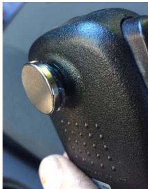
Fig. 1 Hot Glued Magnet on Mic
