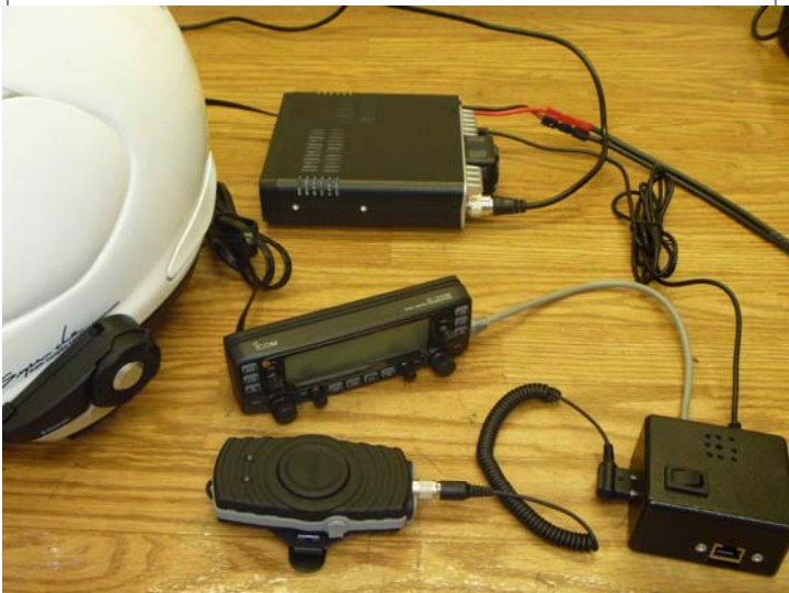
Control Head, PTT Button for Handle Bar, Helmet containing mic and earphones
