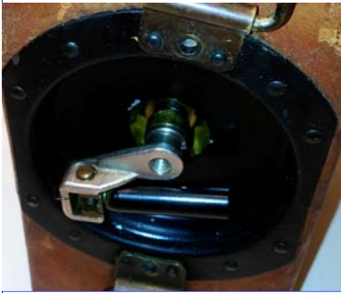
Fig. 21 American phone's self-retractable crank handle
