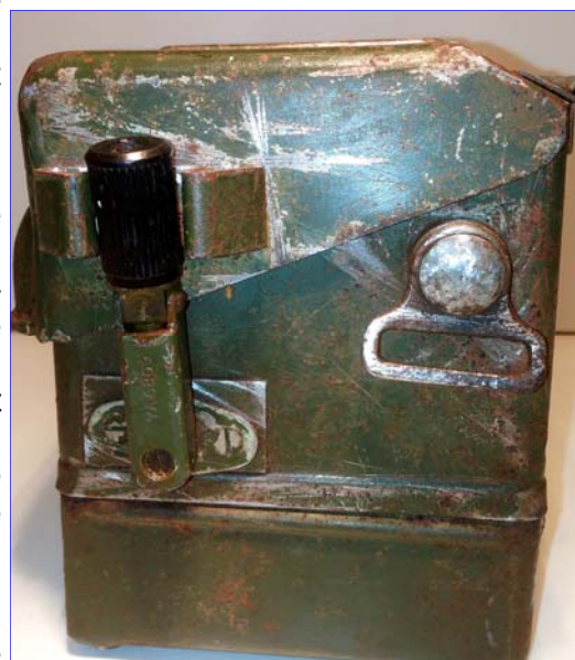
Fig. 20 British phone's crank handle rest
