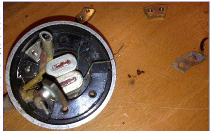
Fig. 16 Damaged Japanese headset receiver
