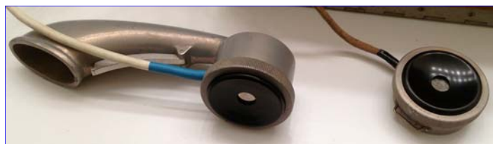
Fig. 19. Japanese Type 92's handset and a sub-receiver
