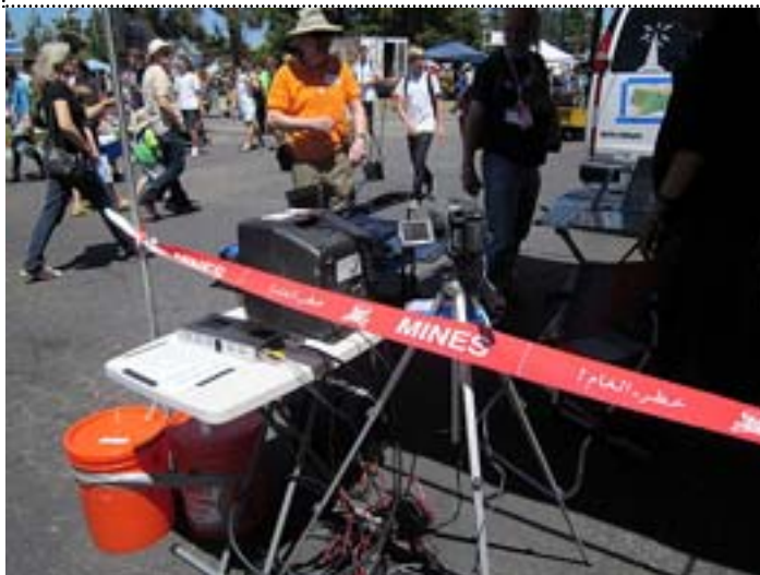
Amateur TV setup is receiving transmission 427 MHz (CATV ch 58) from inside Expo Hall at booth 89
