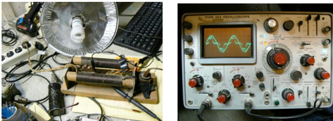
Figure 6. (a) Setup for testing CFLs; (b) measured waveforms [Korsak].
