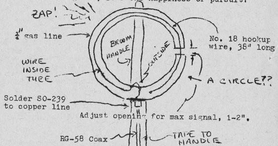
Antenna is unidirectional. (really?) Maximum signal occurs with open side toward signal. Null is with the closed side towards signal.
